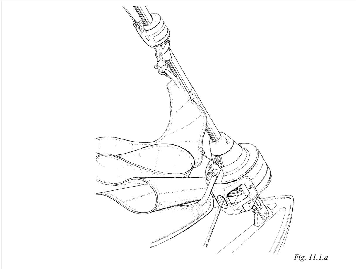
5. Attach the sheet to the clew. Take the sheet through the lead block and then on to the cockpit. Put a figure-of-eight knot in the ends.
