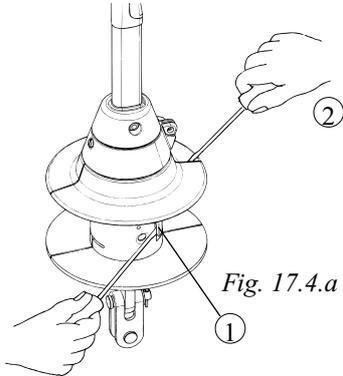
Insert a screwdriver ① under one of the connecting clips. At the same time, press another screwdriver ② between the drum halves on the same side so that these are forced apart 3–4 mm.
