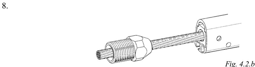
Thread the socket onto the wire.
