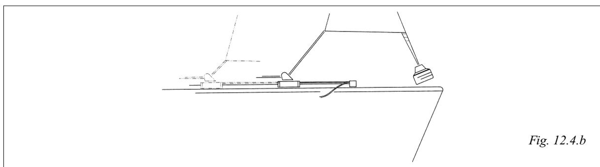
Many furling foresails have markings in the foot for different reefing positions. After you have tested combinations of sail area and sheeting position to see which function satisfactorily, you can use these markings as a reference and mark suitable sheet points on the track.
