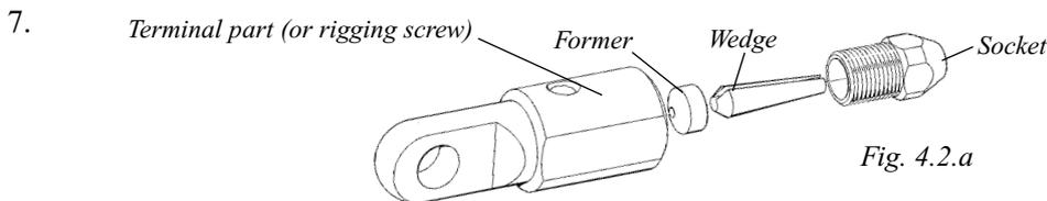
Unscrew the socket, wedge and former from the terminal part (or Furlex rigging screw if to be used.)
