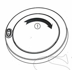
1, Gently apply firm pressure against the Lens and turn cleckwise to loosen.
