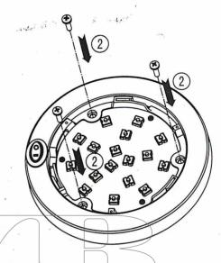
2, Install the Base by fastening 3 screws in place.
