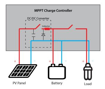
MPPT controllers do this via an adaptive algorithm that follows the maximum power point of the PV array and then adjusts the incoming voltage to maintain the most efficient amount of power for the system.
