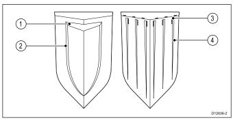
Air trapped under the front of the vessel can travel under the hull and appear as aeration.
