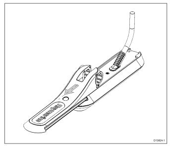
The transducer is now ready for attaching the accessory bracket.
