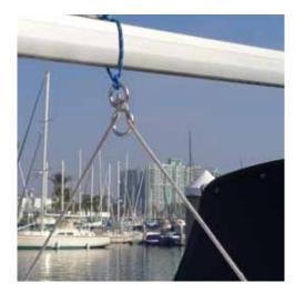
"The simple boom brake" This boom rappelling device uses different degrees of friction to slow down the boom swing when jibing. Method reduces the slamming of the boom from side to side. This is done by allowing the boom to shift while being restricted by the amount of friction rigged into the TackRite rappeler. Attach the TackRite rappeler device to the boom with  $\frac{1}{2}$ " line.
