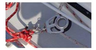
A block can be added to one of the cleats allowing rappeler line to lead back to a cockpit location for additional control.
