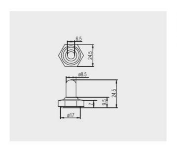
Neopren®- cap for screwing on (M12 x 0.75) to levers of the series 1820 for dust and water protection of the actuator side
