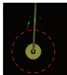
MOB indication on the radar screen
