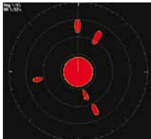
An example of Main Bang interference on a 4kw radar screen
