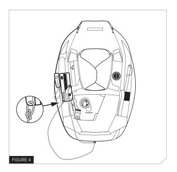
Double check to see that the orange arming tab is still hanging loosely and repack the PFD as per the Owner's Manual. Make sure that there is nothing that will tangle or stop the lanyard from pulling the red cap off when the PFD inflates.
