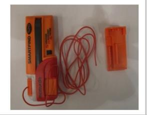
5) Attach the S20 unit (a) to the crocodile clip (b) by sliding it down the recess until an audible click is heard.
