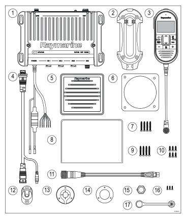
Ray90 / Ray91 VHF DSC Radio base station (including fitted power and data cable).
