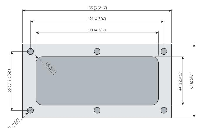
\*Use actual bailer as a guide for location of holes to be drilled.
