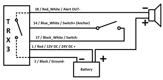
Figure: 5 Anchor Alert connection sketch
