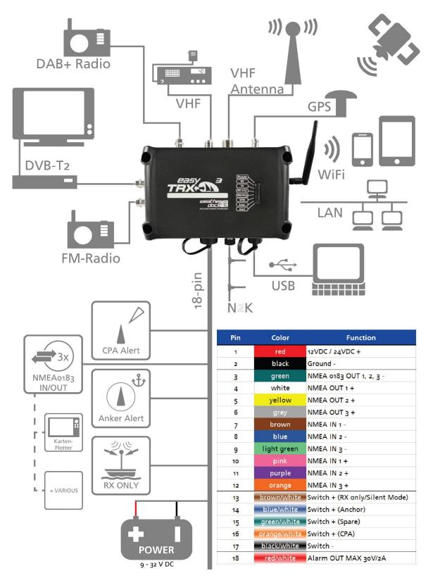
Figure: 3 Connection possibilities and cable colors
