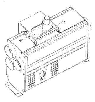
And Lock the device with the mounting bolts.
