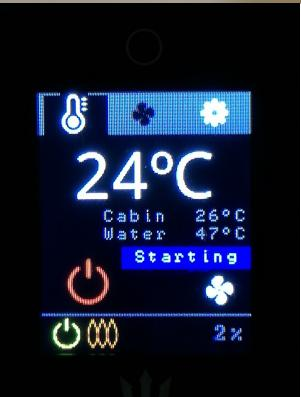
When burner ignites, the flame indicator light is turned on.
