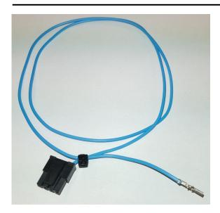
If the heater is needed to be shut down from the boat's main switch, use the spare part **363640** to the heater, and connect the another end of the wire to the main switch. The heat will not start without turning the switch **ON**, and it will perform a controlled shut down when the switch has been turned **OFF**.
