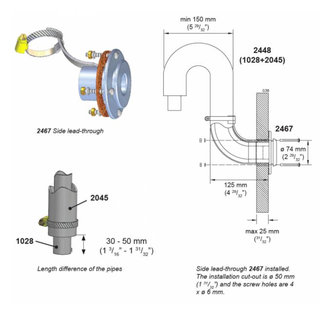
A side lead-through is installed in the side of the boat or in the transom. In sailboats it is recommended to install it in the transom. The installation always requires a so-called goose neck piece. Make the necessary installation cut-outs and spread a suitable sealing agent on both sides of the seal and on the screw holes. This will ensure that the connection is waterproof.
