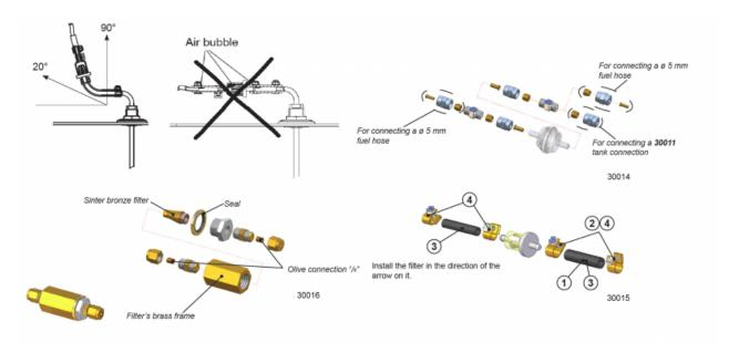
Filters can be installed in a ø 5 or ø 6 mm plastic tubing or 1/8" metal pipe. Ensure that the fuel pipes are clean before installing the filter. There must be no debris or impurities between the pump and the filter as they will clog the pump. The filter type must be selected according to the operating conditions and country-specific requirements.
