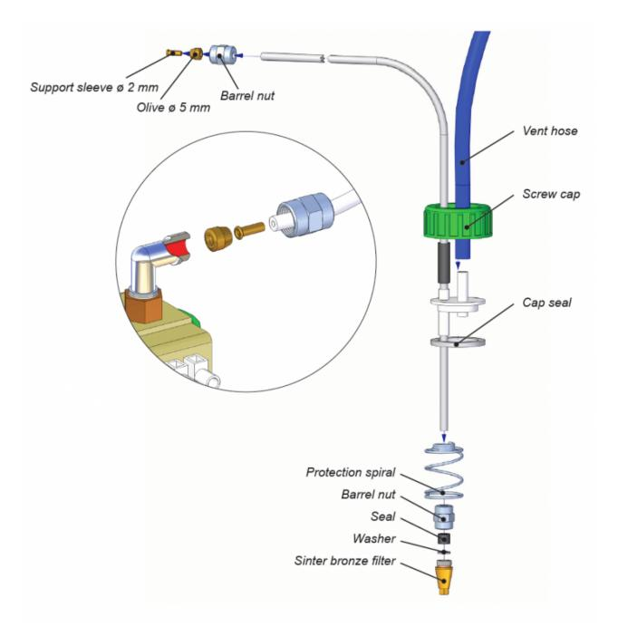
If the fuel will be taken from a separate Wallas day tank, you must install a tank connection 367215 (4 m) / 367216 (6 m).
