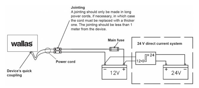
Electrical connections of the device
