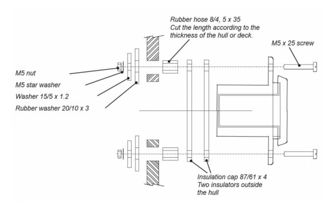
Insulation kit for a metal-hulled boat
