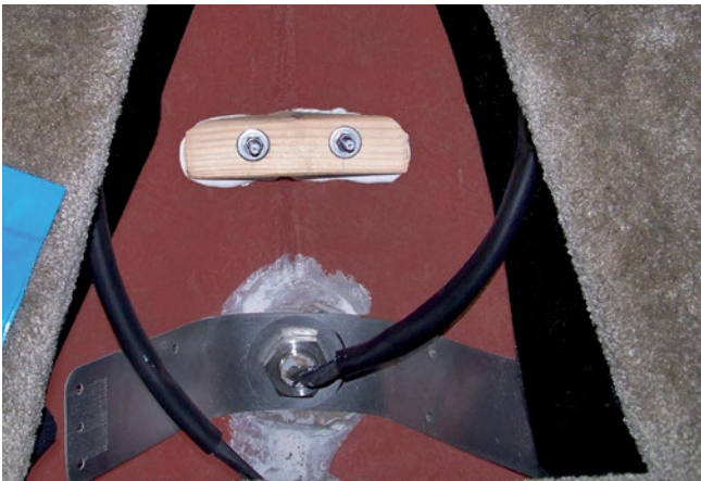
Fig. 25: Screw connection GRP in the boat interior
