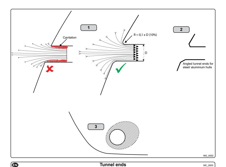
Rounded tunnel ends will maximise thrust and minimise noise and cavitation.
