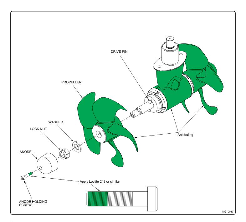
Propeller Installation MC\_0018
