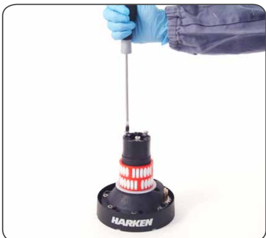
6. Completely unscrew the three screws n° 27
