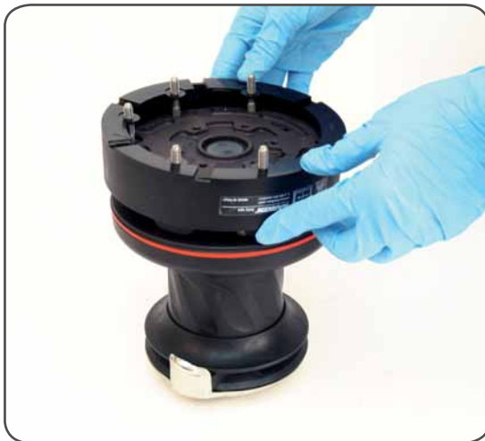
4. Reposition the skirt n°2 in its housing
