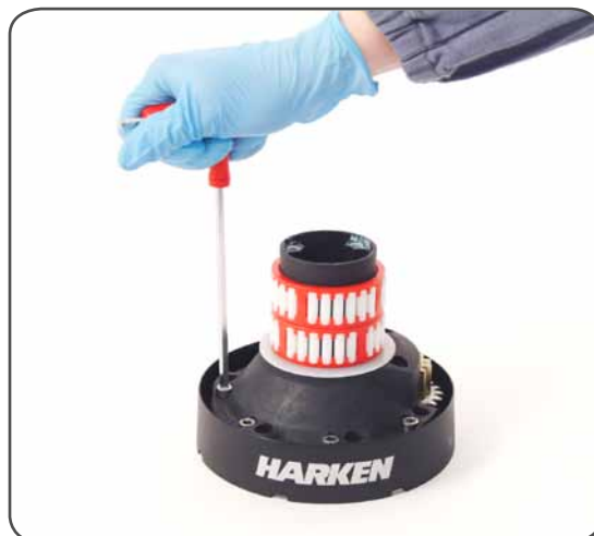
7. Remove the self-tailing arm support n°21
