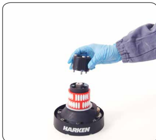
7. Remove the self-tailing arm support n°21
