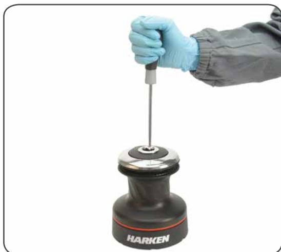
1. Unscrew the central screw ( \curvearrowright 2Nm/18 in-lb)
