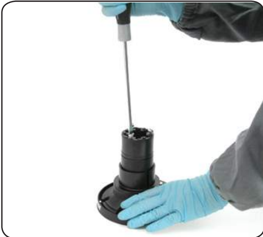
6. Completely unscrew the three screws n°18
