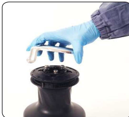
4. Remove the self-tailing arm n°17 by rotating and lifting it.
