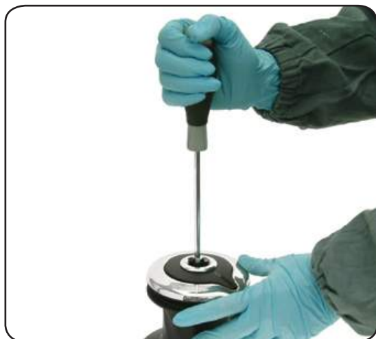
1. Unscrew the central screw ( \approx 2\text{Nm}/18\text{ in-lb} )
