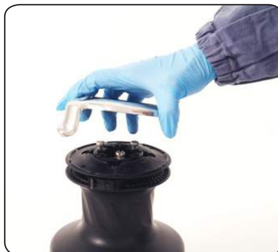
4. Remove the self-tailing arm n°28 by rotating and lifting it.
