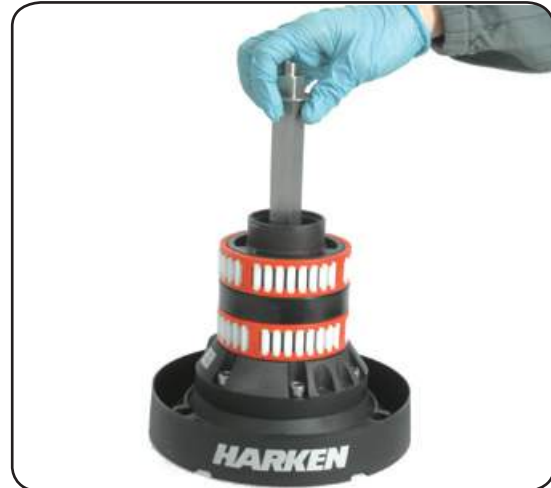
7. Slide out the central shaft n°21
