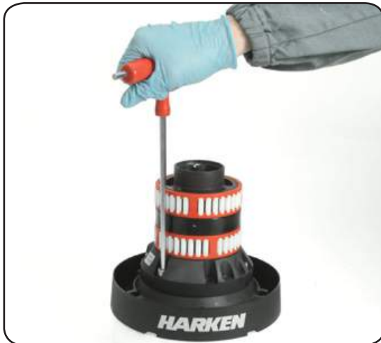
8. Unscrew the 5 hex screws n°18 ( \approx 20\text{Nm}/177\text{ in-lb} )
