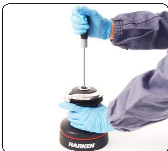
1. Unscrew the central screw ( \approx 2\text{Nm}/18\text{ in-lb} )
