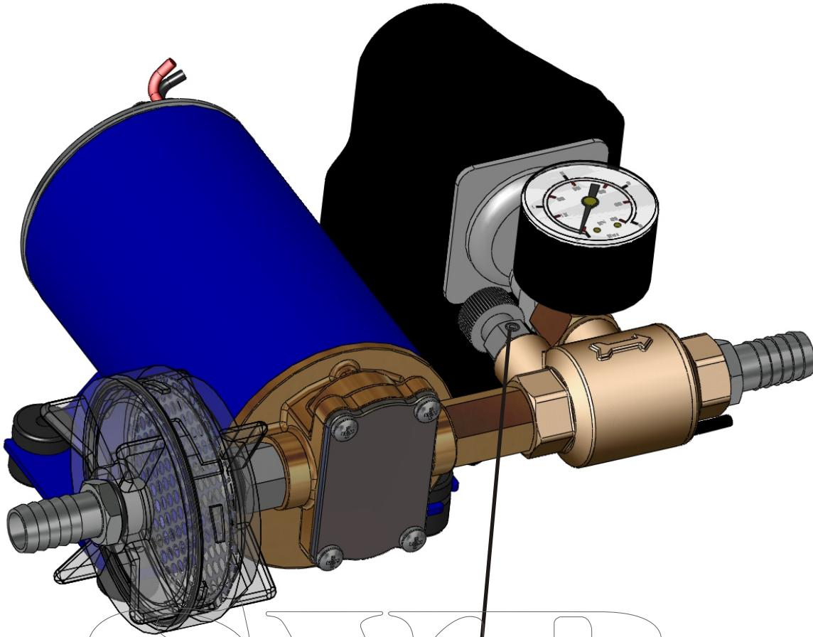
When starting the pump slightly open the small valve located next to the pressure switch, in order to let the air out and facilitate the pump priming. As soon as the pump is operating close the small valve.
