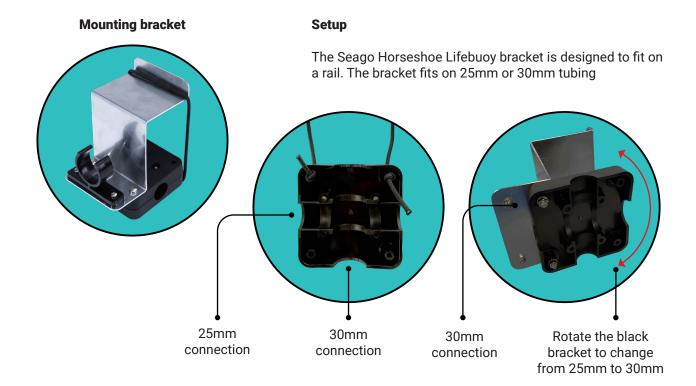
The black plastic rail mount bracket is ready to install on a horizontal 25mm rail. If you require the bracket to mount on a 30mm horizontal rail you will need to:
