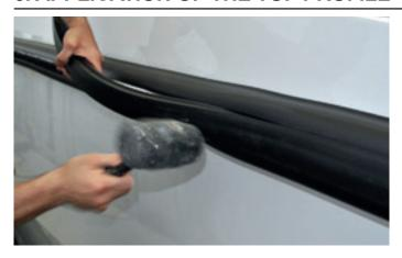
Install the top profile by pressing it with a rubber hammer.
