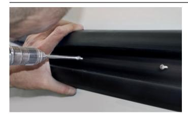
Drill and screw the base profile directly to the boat.
