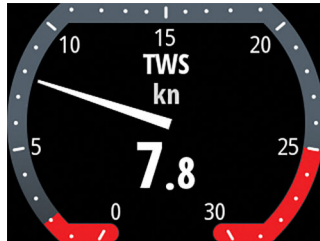
True Wind Speed page showing high and low true wind limits
