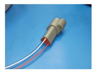
**Step 6**: From the front side insert secure tab. This prevents crimp contacts to fell out of connector housing.
