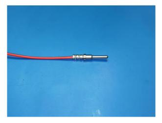
**Step 4**: Insert three crimped pins into connector on dedicated place. Make sure pins are secured, test them with slight pull outwards. Take care not to mix pins functionality.
