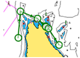
Result after automatic routing
