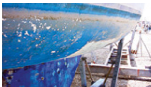
Paint blisters and lifts
