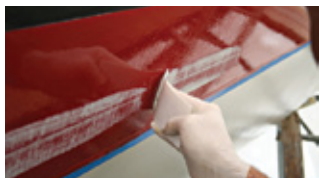
Fill along boottop
