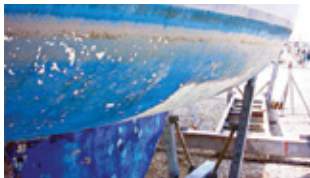
Paint blisters and lifts
