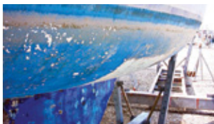
Paint blisters and lifts
